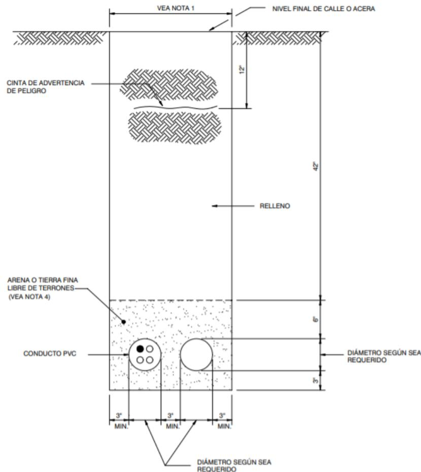
Figure III-2 – Typical Underground Conductor Installation
