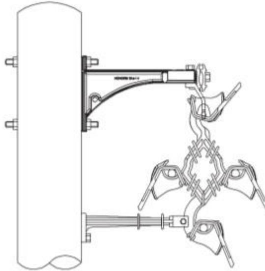
**Figure III-1 – Triangular Cable Spacer Bracket** (source: Hendrix Aerial Cable Systems)
