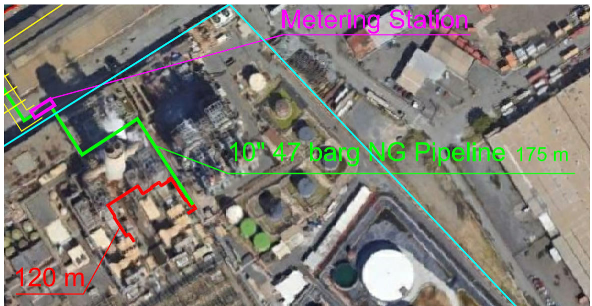
Exhibit 23: Gas line from Metering Station to turbines
