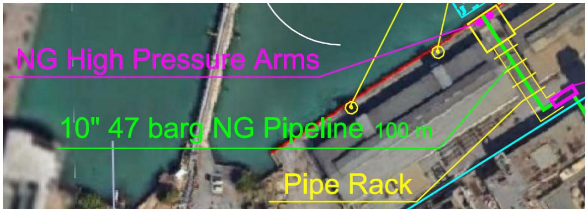
Exhibit 21: Detail of the aerial pipe rack
